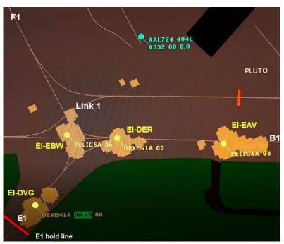
**Image No. 1**: Labelled A-SMGCS image of Link 1 showing the relative positions of each aircraft
